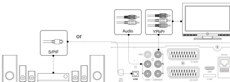
**NOTE :** When you have an A/V receiver with S/PDIF digital audio input, this connection is recommended to enjoy the best audio quality, especially for the Dolby Digital sound.
